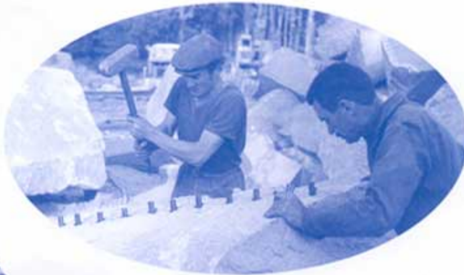
Cutting of granite head with 22 x 115 wedges
